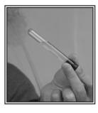
7. Invert or shake the test tube to dissolve the tablet.
