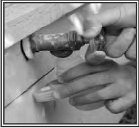
**1.** Turn on the tap and fill the sample bottle. Use a different (labeled) sample bottle for each house. If it is raining, take precautions to ensure that no rainwater enters the sample.
