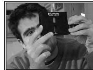
**9.** Insert the test tube into the reader. Hold the reader so that a light-colored surface like a wall is behind it, but do not hold it to a light source. Match the color in the test tube to the closest color on the color slide. If the color in the test tube is between two colors on the slide (for example, 6 and 8 ppm), record the number which falls in between (in this case, 7 ppm).
