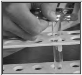
**4.** Add one tablet of Nitrate #1 reagent (labeled on back of packet) to the test tube. Insert the rubber stopper.
