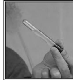
**7.** Invert or shake the test tube to dissolve the tablet.
